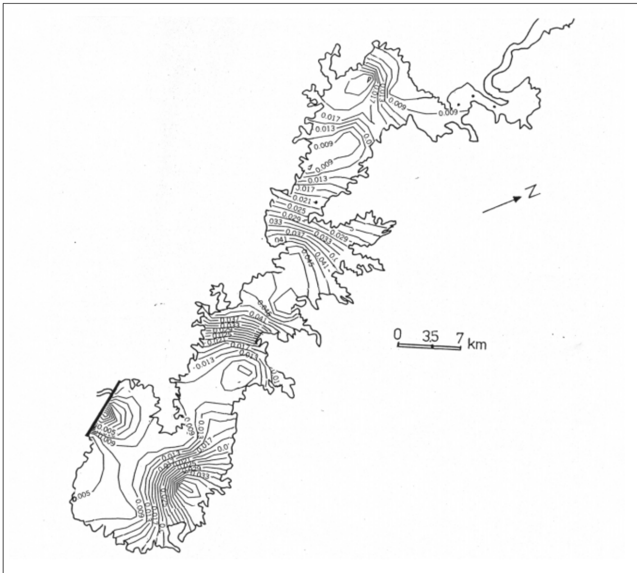
Figure 7. Iso contour line for the D_{50} of the bed sediment of Mosul Dam reservoir.
