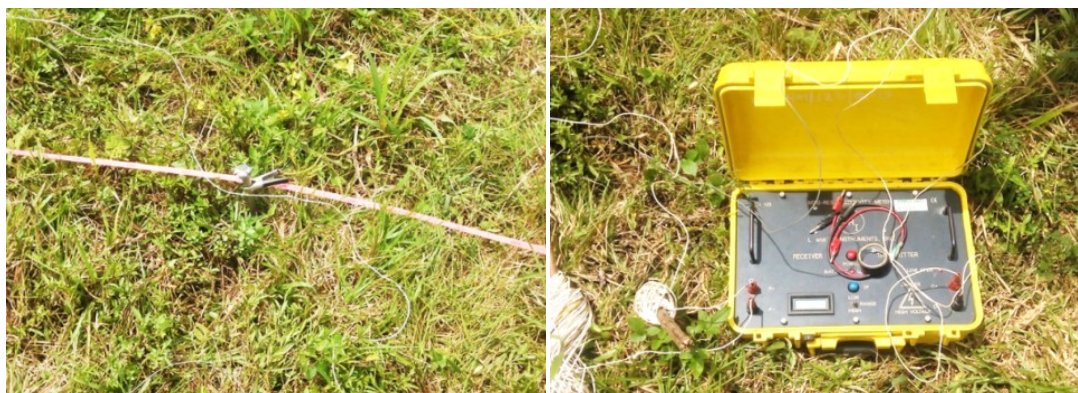
Plate 1. Electrical Resistivity Profiling with Minires Resistivity Meter
